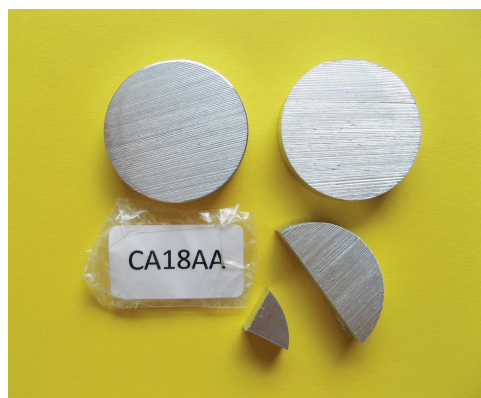
Titel: Interlaboratory comparison for proficiency testing CA18AA chemical analysis of an aluminium alloy (wet-way analysis)
